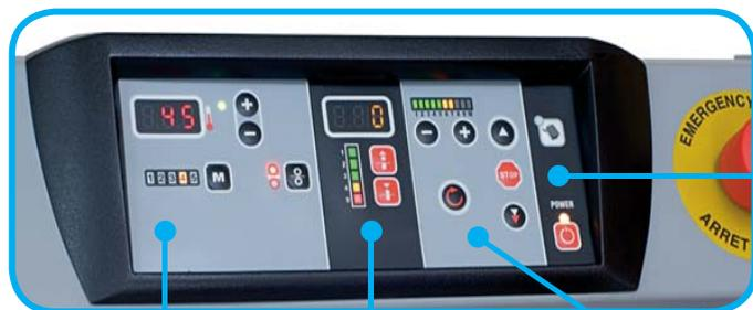
Foot switch selection and power button (when switching the machine off, the upper roller automatically lifts up in order to preserve the rollers).
