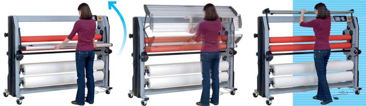
The feeding tray pivots upwards leaving a full and secure access to the machine when loading the film. In upper position, the driving motor is shut, preventing the operator from any injury during the operation.
