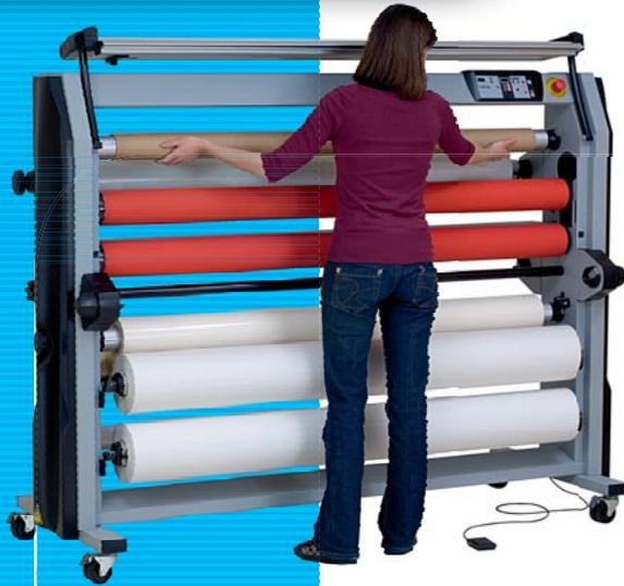
With our new even lighter self-blocking roll-shafts, you will save time while changing film. No tools are required unlike systems using locking rings or pivoting shafts needing a large space behind the machine.
